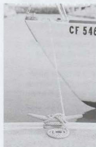
Cleated docking lines should always be secured with a cleat hitch
