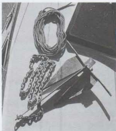
The Danforth anchor is very common. It is strong, lightweight, holds well, and is easy to store.
