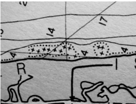
This chart detail shows the symbol for rocks that lie underwater at all stages of the tide.
