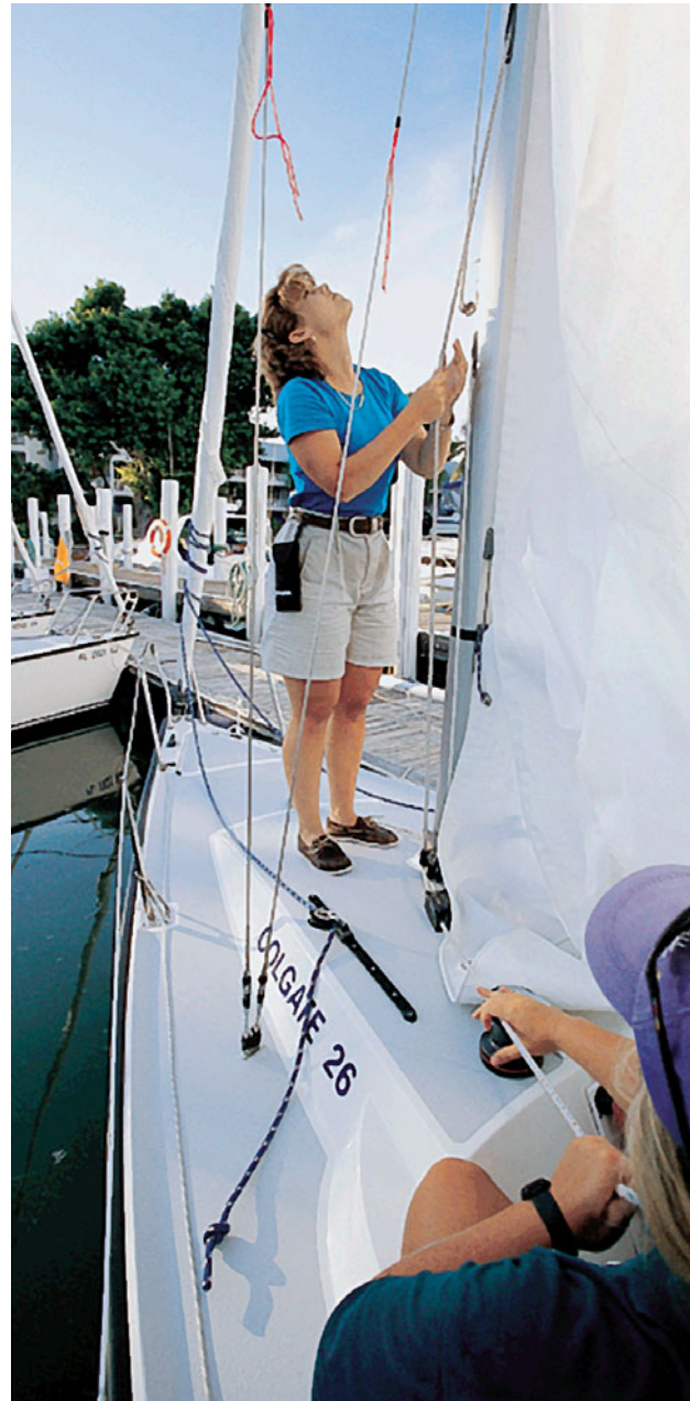
Figure 1-5. Raising a sail with the halyard (running rigging).
