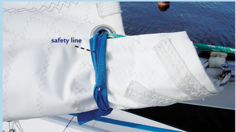
C. When settled down, tie a safety line
