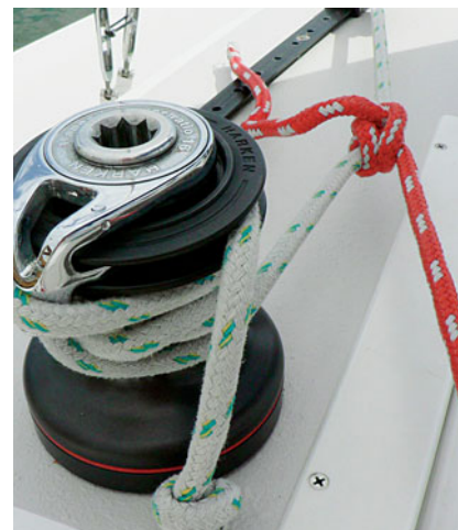
Figure 10-5. Using a spare line, tie a rolling hitch to the line that is jammed on the cleat to relieve the strain, then untangle the wraps on the winch.
