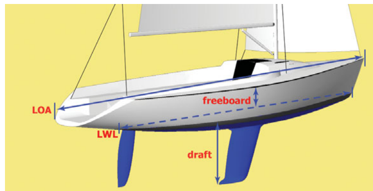
Figure 1-1. Terms that describe a boat's dimensions.
