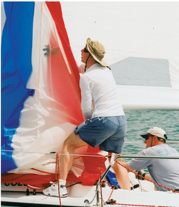
Figure 9-6. Douse the spinnaker quickly and smartly, stowing it off the deck as quickly as possible.
