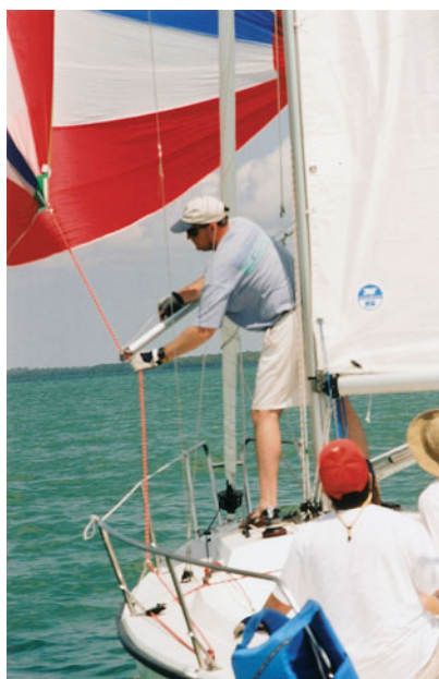
Figure 9-3. Next attach the end of the pole to the old sheet. (The line that was the sheet becomes the spinnaker guy.)
