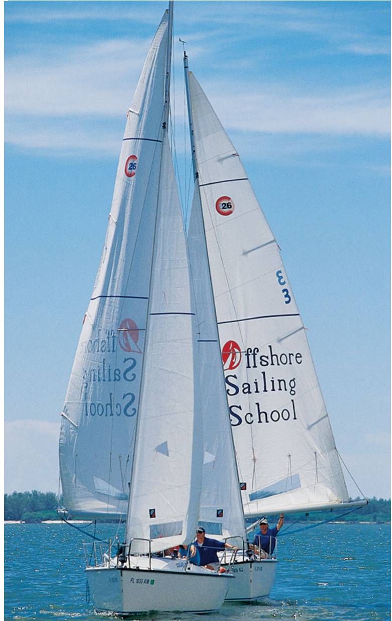
Figure 4-23. Sailing by the lee, with the wind on the same side as the boom, this boat is in danger of jibing.
