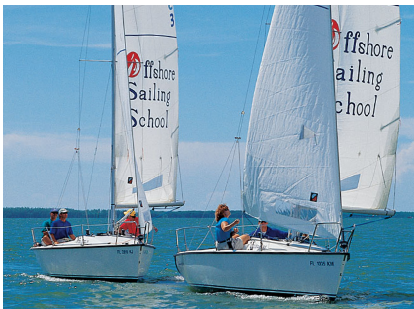
Figure 4-9. The jib on the boat behind is blanketed by its main, while the lead boat sails wing and wing.
