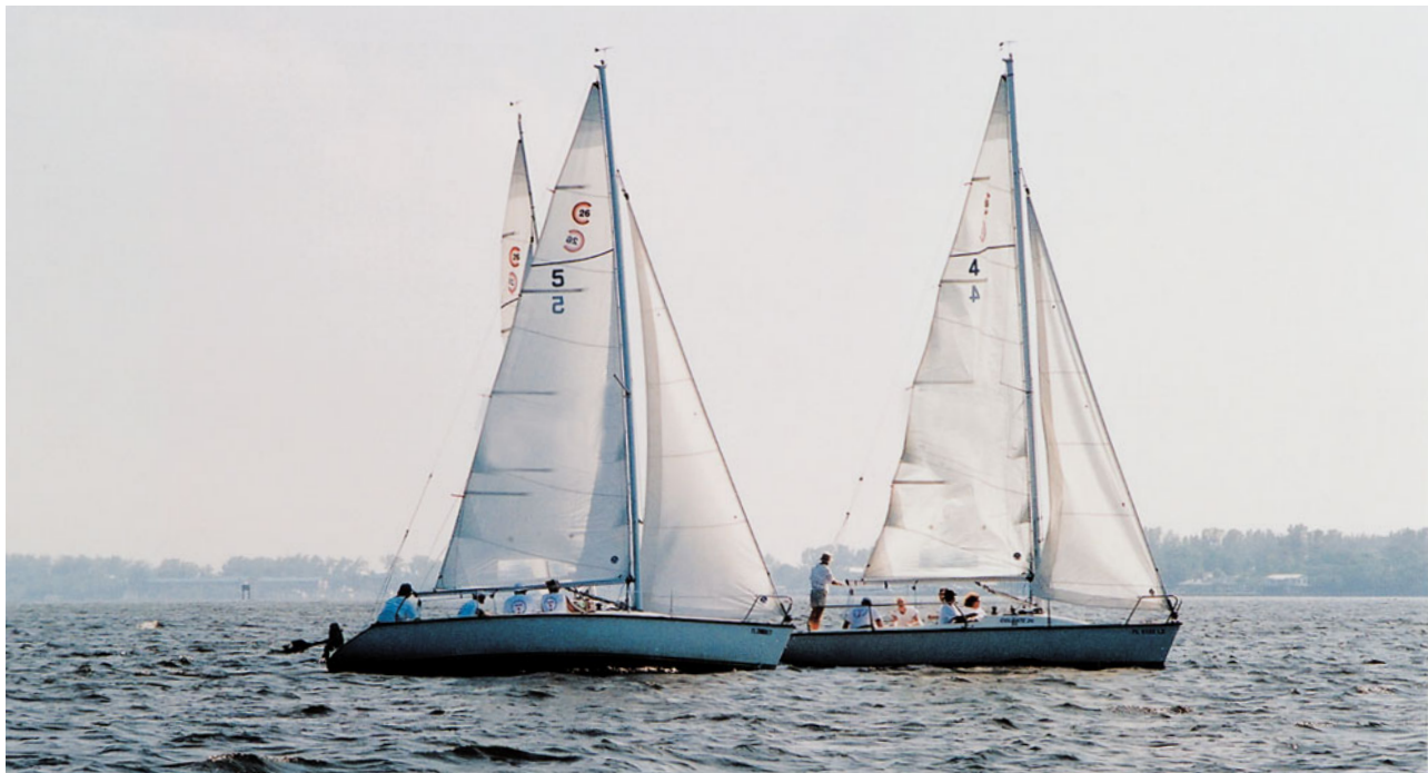
Figure 3-14. The lead boat is head to wind, and its sails are luffing; the boat behind has trimmed sails.
