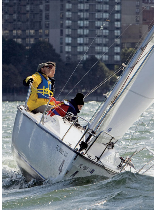
Figure 5-4. As a boat heels, the leeward bow wave pushes the bow to windward.
