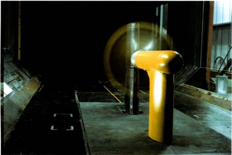
Plate 1 Arrangement of rudder-propeller rig in wind tunnel (See also page 129 of this book)
