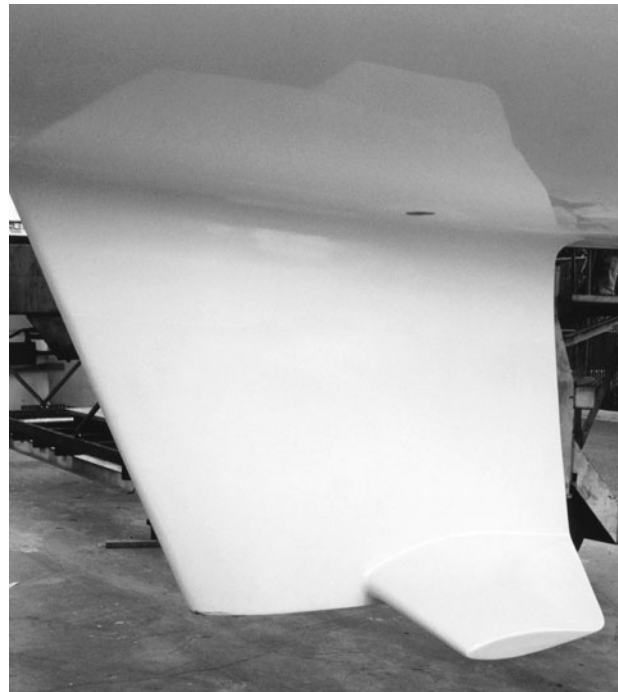
With help from Dave Vacanti I designed a wing keel for the Islander 34 to provide a shoal-draft option. This configuration worked exceptionally well in two days of boat-on-boat testing against a deep-draft version.
