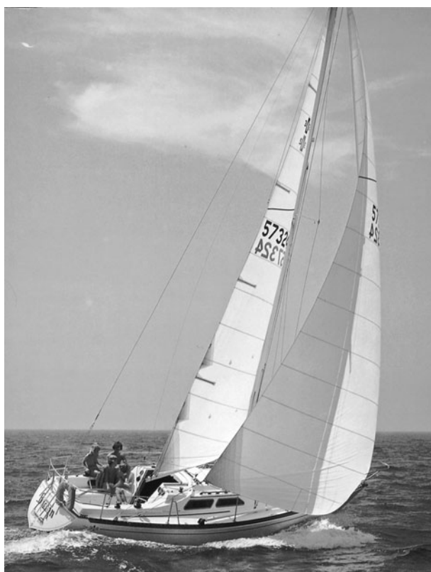
This photo from Islander's first brochure for the Islander 32 shows a genoa that is way too large by today's standards, but that's the way we did it back then. The genoa lead car is way aft, adjacent to the sheet winch.
