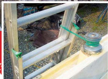
(top). The scene of the accident, a long way to fall. (inset) Bungee tied to a winch prevented the ladder from kicking completely out and dropping me to the ground.
