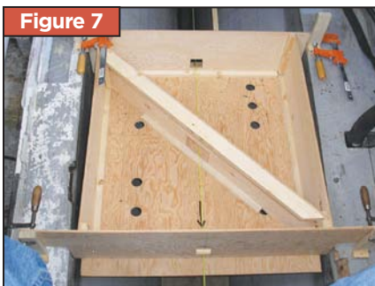
Figure 7 Template for locating the new engine mounting brackets.
