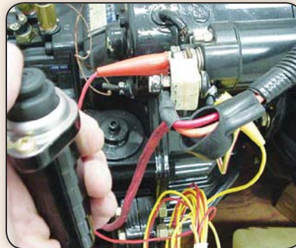
Remote starter switch connected to starter solenoid.
