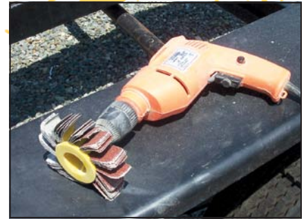
All the reason you need for proper eye protection. Those flapper wheels throw dust and debris as well as an occasional flap.
