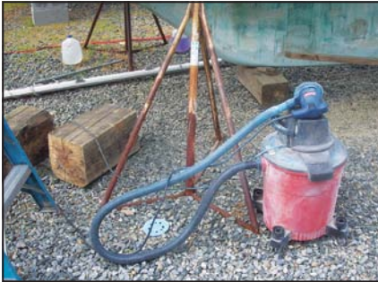
Proper set up for sanding: eye protection, respirator, bunny suit and a shop vac for dust.
