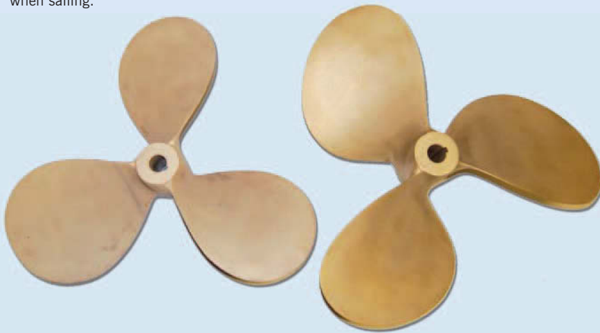
The “round” or symmetrical, three-blade, fixed propeller on the left provides better performance in reverse than the asymmetrical prop on the right. This powerboat design, however, works better in forward and is most commonly available.
