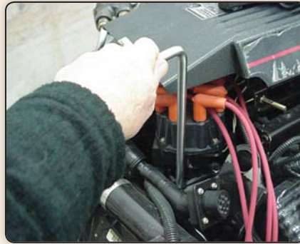
Using a distributor wrench to adjust base timing.
