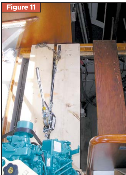
Figure 7 Template for locating the new engine mounting brackets.
