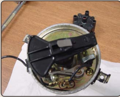
Distributor shows rotor points and condenser mounted to breaker plate.
