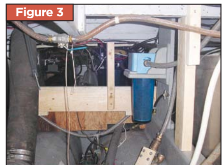
Typical temporary cabin sole support.
