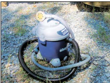
(top) A close up of the sander/shop vac setup. This older model has several problems, it's very noisy and the hose doesn't lock in the canister. (bottom) A newer shop vac is worth the expense. It's quiet and the hose locks in the canister, keeping it from pulling out at the wrong time.
