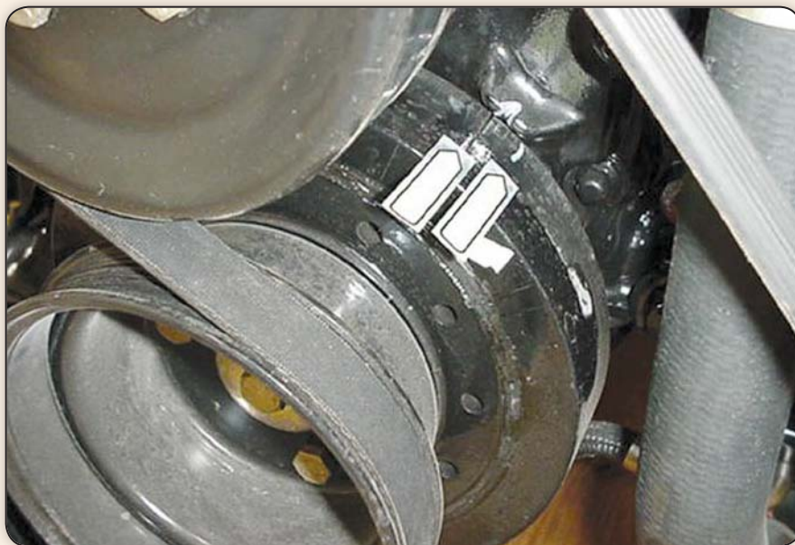
Timing marks on a GM 350 CID engine.
