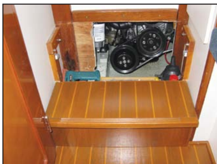
(top) Completed steps. (middle) Traction grooves routed into the edge molding. (bottom) Top step and riser remove for access to storage and the engine.
