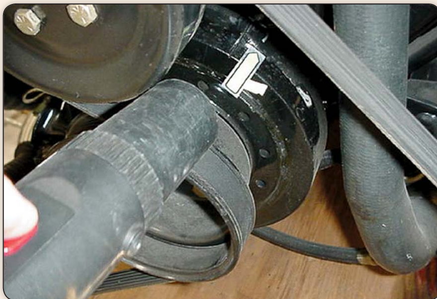
Checking base timing with a timing light.
