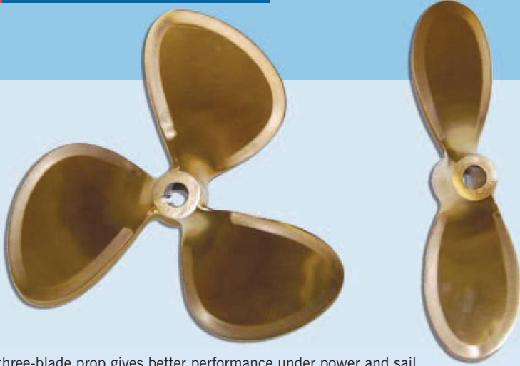
The three-blade prop gives better performance under power and sail but the increase drag can reduce boat speed as much as 1.5 knots when sailing.
