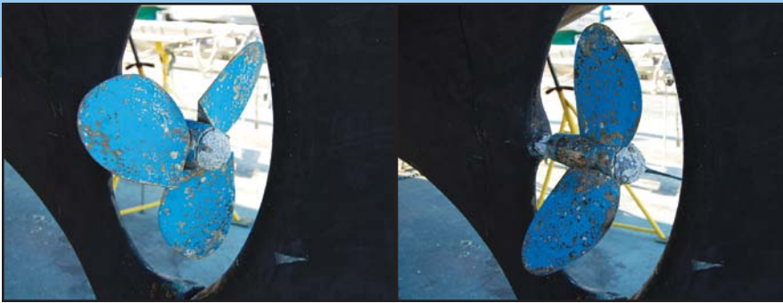
(left) A three-blade, feathering propeller in the sailing position. Note how the top blade lines up behind the keel. (right) A three-blade, feathering propeller opened up in the power position.
