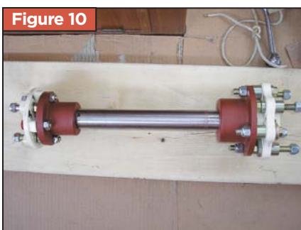
Figure 10 New shaft extension with R&D flexible couplings installed.
