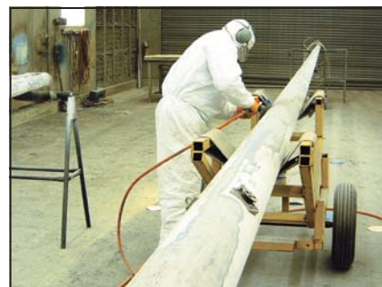
Paint that is flaking or pitted is stripped to bare metal by sanding with 80 grit hook and loop 5" (127mm) discs on a dual-action air sander. Sound areas are thoroughly sanded with 220 grit.
