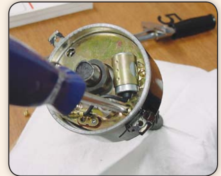
Removing the breaker plate.
