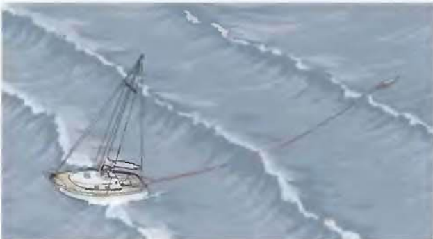
Drogues help prevent broaching and twisting sideways onto the waves.
