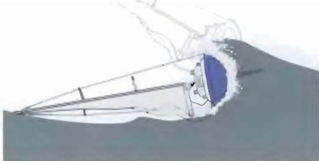
A breaking wave the same height as the beam can capsize the boat.
