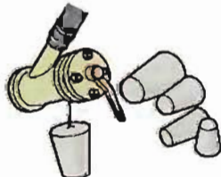
Working seacocks with emergency softwood sealing bungs to plug broken skin fittings
