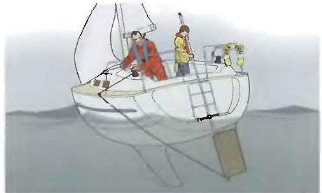
Jury rig a steering oar using the spinnaker pole and washboard or cabin locker cover.
