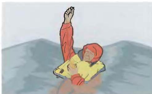
The MOB should hold the antenna as high as possible to give the greatest range.
