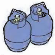
Gas kept in a properly vented locker with all pipes and connections regularly checked for leaks
