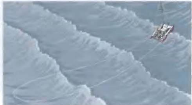
A long loop of trailing warp can also be used in a following sea.
